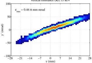
Figure 4. ISDR vertical emittance plots without and with krypton.
