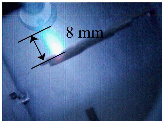
Figure 6: Plasma plume from the target (30 Hz repetition rate).
