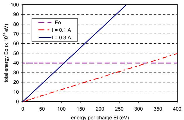
Figure 1: Comparison of the ion beam energy and of the the plasma ions energy content.
