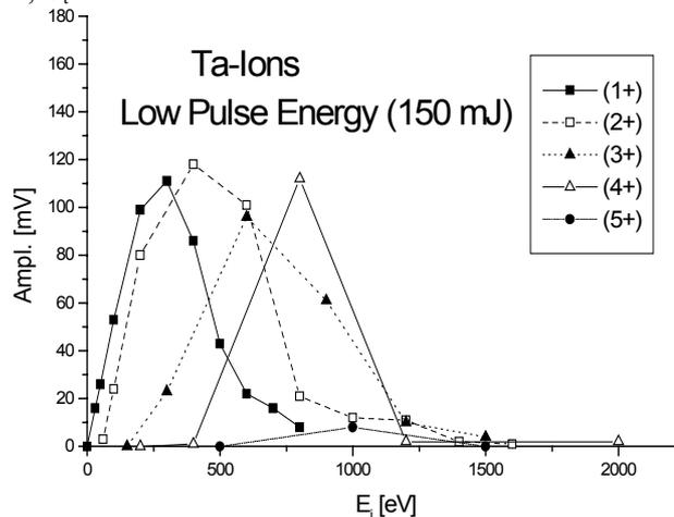
Figure 4 A typical IEA spectra for a laser pulse of 150 mJ irradiating a Ta target at LNS.
