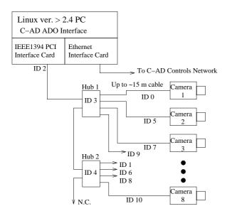
Figure 1: IEEE1394 Camera configuration for a single host. ID's are physical id's assigned by the bus.
