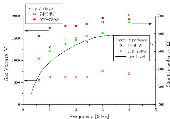
Fig.4: Gap Voltage and Shunt impedance in 6 cores. Squares and circles indicate the gap voltage and the shunt impedance, respectively. The solid line indicates the result from the low-level test on the shunt impedance.
