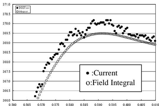
Fig. 3: Tracking between the excitation current and the field strength in dB/dt = 3.0 T/s just before a flat top. The open and closed circles indicate the integral field and the excitation current, respectively.
