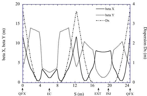
Fig. 2: Lattice functions of the S-ring in the superperiodicity of 1.
