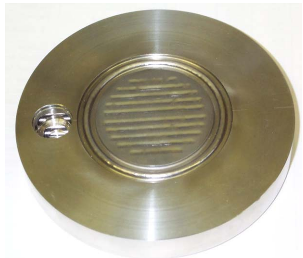
Figure 4: Beam absorber, view from proton beam side.
