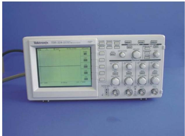
Fig. 6: TDS-224 4-channel digital oscilloscope
