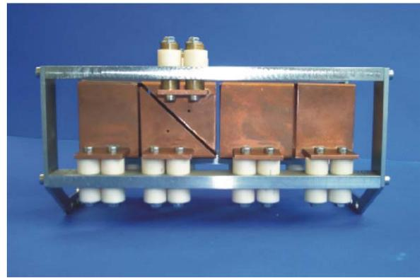
Fig. 5: Electrostatic Pick-Up
