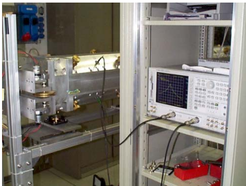
Figure 1: Experimental set-up for the bead-pulling measurements
