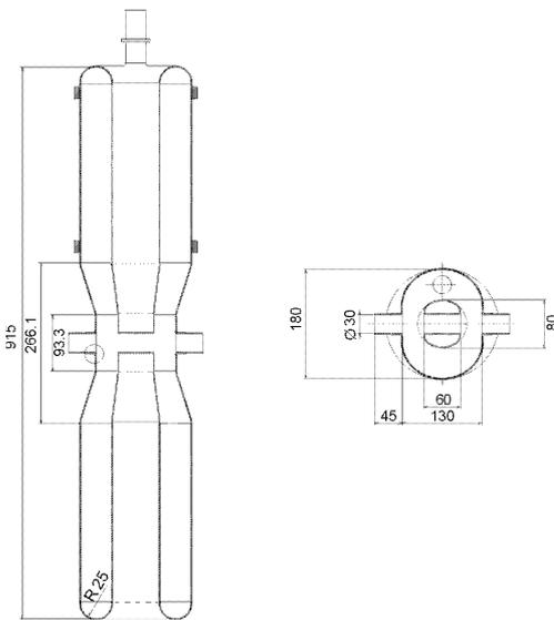
Figure 2: Geometric layout and basic dimensions of the 320MHz HWR
