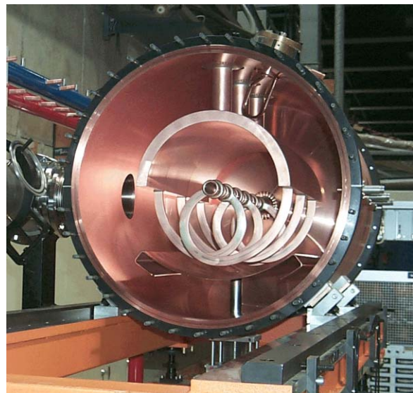
Figure 2: View into a 7-gap resonator.
