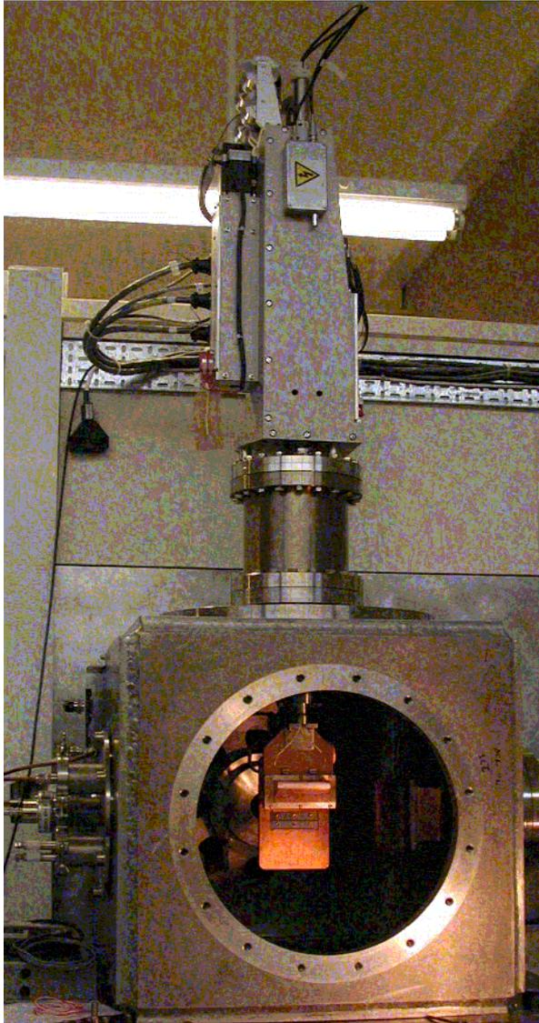
Fig 2 Scanner mounted in ion source test stand.
