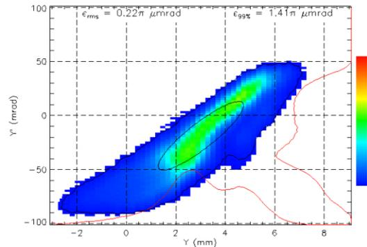
Figure 2: Vertical phase space in LEBT at 35 keV. Gas flow restrictions in place.
