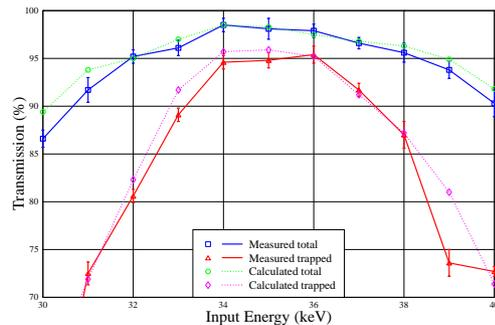
Figure 6: Measured and calculated RFQ transmission efficiencies for total and trapped beam as a function of input energy.
