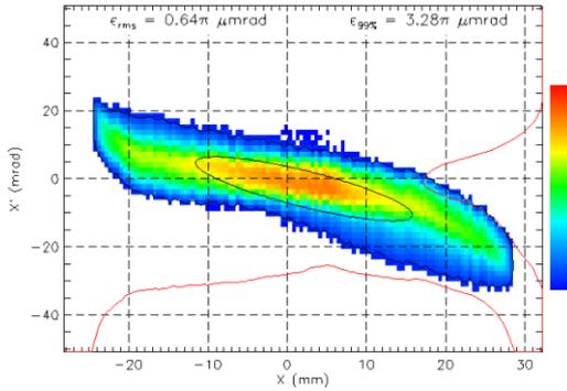
Figure 3: Horizontal phase space in LEPT at 35 keV. Gas flow restriction removed.
