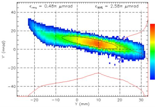
Figure 4: Vertical phase space in LEPT at 35 keV. Gas flow restriction removed.
