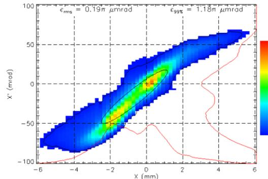
Figure 1: Horizontal phase space in LEBT at 35 keV. Gas flow restrictions in place.
