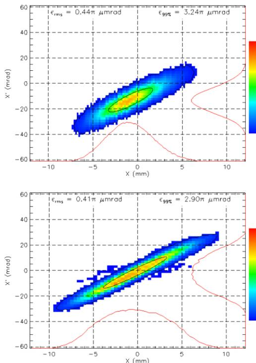
Figure 7: RFQ horizontal output phase space. Top: measured,  $\epsilon_H = 0.44 \pi \mu\text{m}\cdot\text{rad}$  rms, Bottom: calculated
