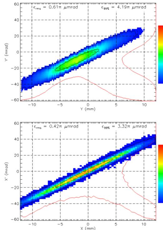
Figure 8: RFQ vertical output phase space. Top: measured,  $\epsilon_V = 0.61 \pi \mu\text{m}\cdot\text{rad}$  rms, Bottom: calculated
