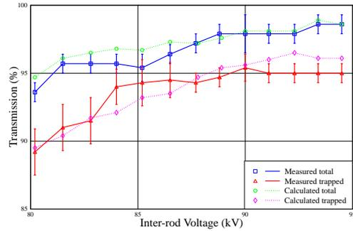
Figure 5: Measured and calculated RFQ transmission efficiencies for total and trapped beam as a function of electrode voltage.
