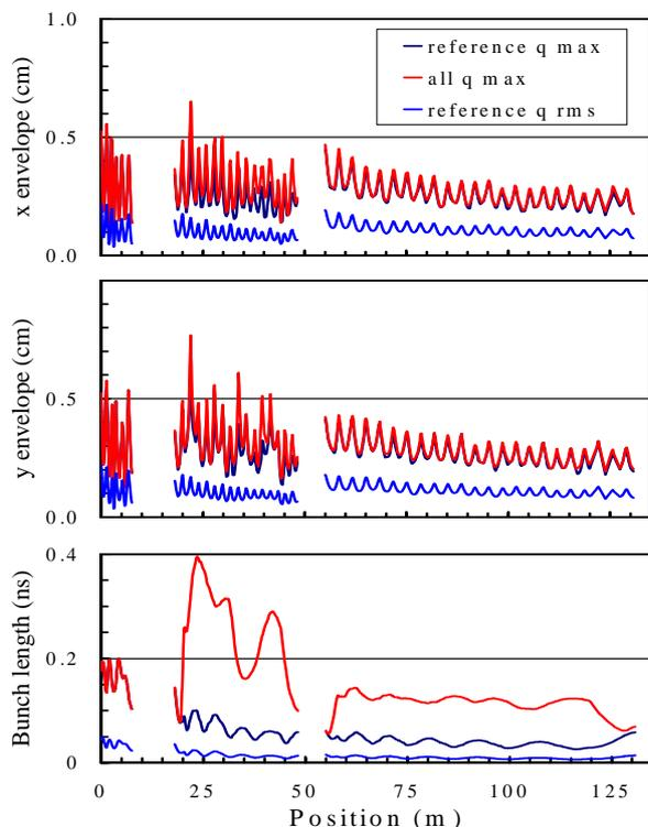
Figure 3: beam envelopes along the three sections of the linac for multi-charge beam transport in the “2-strippers” mode of operation. The reference and the transported charge states ( $q$ ) are given in table 1. The large change in the bunch length after the strippers reflects the multi-charge phase synchronization.
