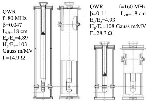
Figure 2: Example of two LNL SC cavities.
