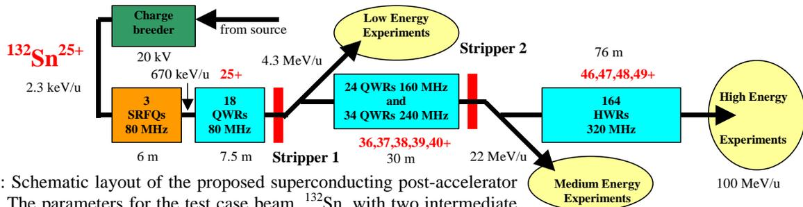
Fig 1: Schematic layout of the proposed superconducting post-accelerator linac. The parameters for the test case beam,  $^{132}\text{Sn}$ , with two intermediate stripping stations, are presented.
