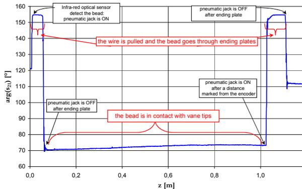
Fig. 4: measured phase for 1 quadrant (E-field)
