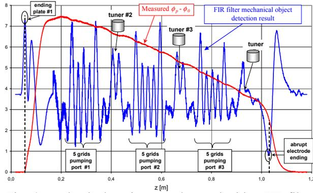
Fig. 6: mechanical equipments detected with a FIR filter
