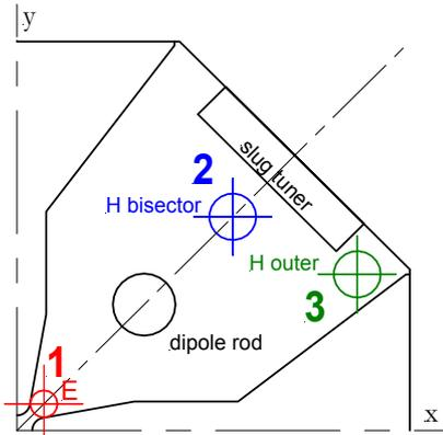
Fig. 2 : 3 tested positions in the transverse section
