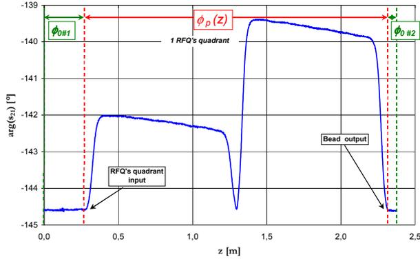
Figure 5: measured phase for 1 quadrant (*H*-field)
