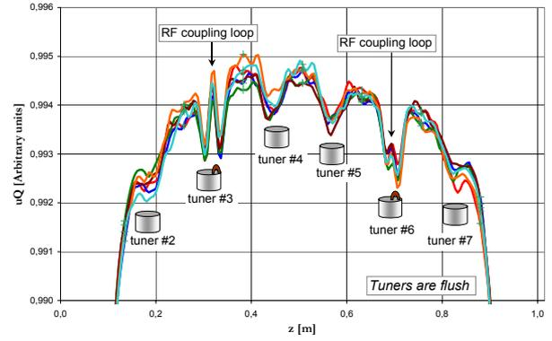
Fig. 7: six aligned and scaled modal voltage profiles
