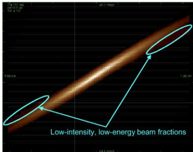
Figure 4: Vertical emittance of a 21.8-mA RFQ beam. The measured rms size of  $0.325 \pi$  mm mrad includes a 65-keV beam fraction that carries very little current.
