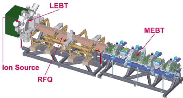
Figure 1: The 9-m long SNS front-end beamline.
