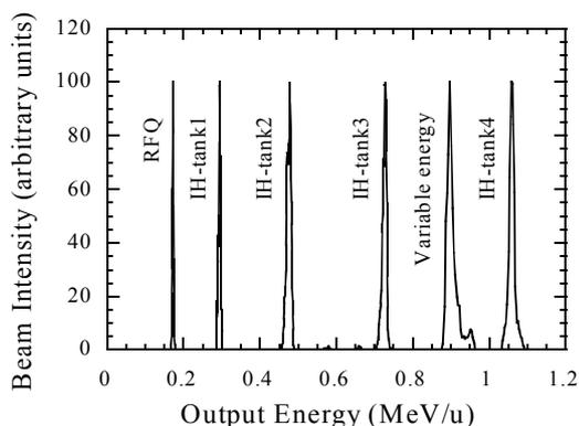
Figure 3: Beam energy spectra under the different operation modes.
