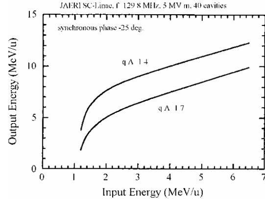
Figure 4: Relation between input and output energies of SC linac.
