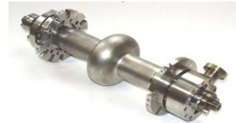
Figure 1: 3 GHz spun niobium cavity.
