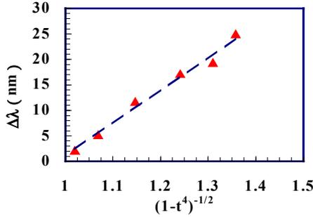
Figure 4: Penetration depth plot  $\Delta\lambda$  vs.  $x=(1-t^4)^{-1/2}$ .
