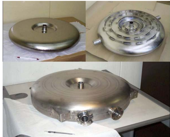
Figure 1. The reentrant cavity in various stages of construction.
