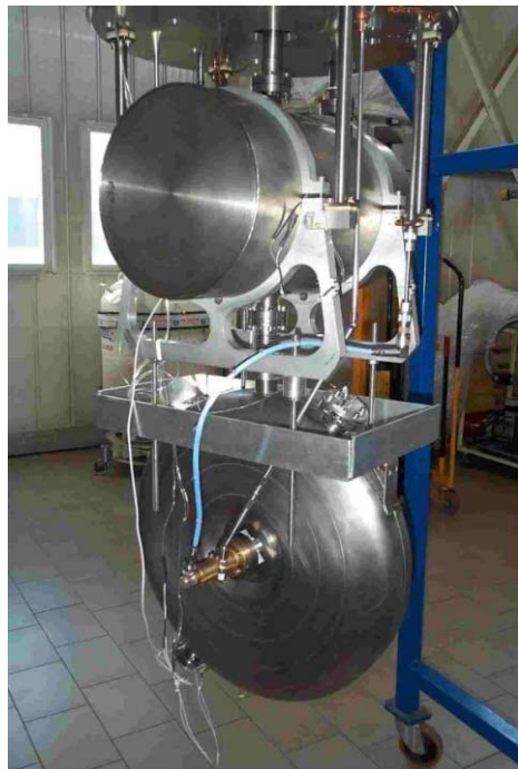
Figure 2. The reentrant cavity assembled in the test cryostat.
