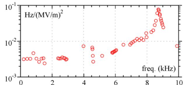
Figure 1 : Distribution of  $K_r$  vs.  $\omega$  for a 9-cells cavity
