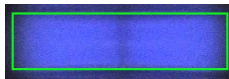
Figure 6: Multipacting induced discharge. The rectangular box outlines the waveguide boundary. The central dark zone is observed for a slotted-waveguide.
