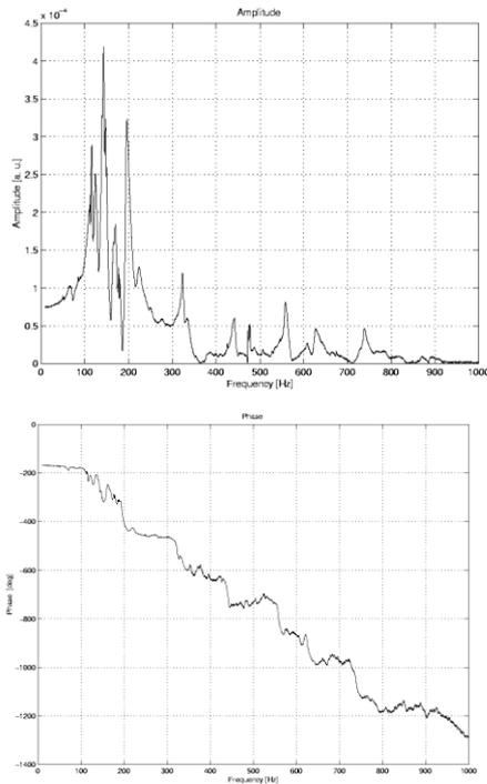
Figure 4: Amplitude and phase signal of the transfer function. Several resonances can be seen.
