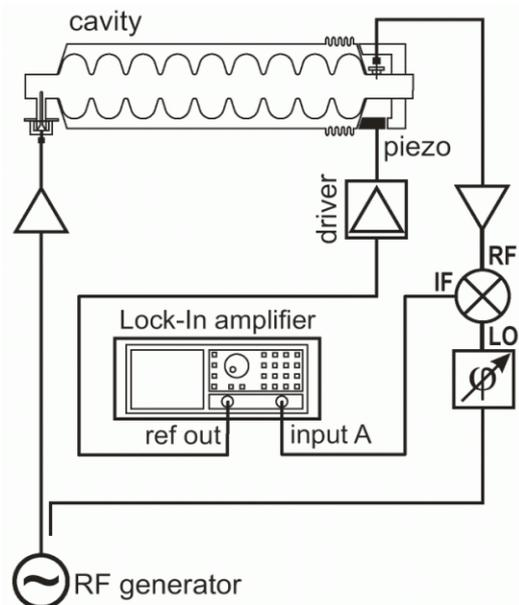
Figure 1: Block diagram of the measurement setup.
