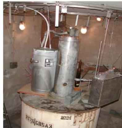
Figure 6: Setup of the cryostat with the Co60 source.
