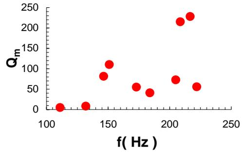
Figure 5: Quality factors for the first 10 dominant mechanical modes of the cavity.
