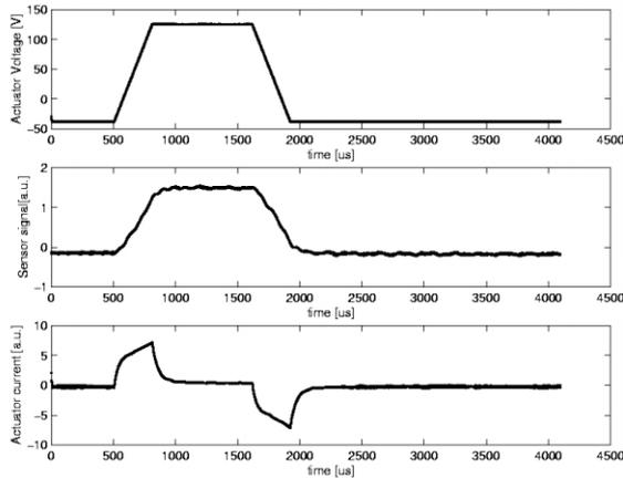
Figure 7: Applied voltage to actuator (top), sensor voltage (middle) and actuator current (bottom).
