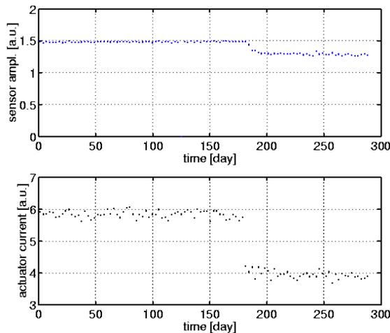
Figure 8 Sensor voltage (top) and actuator current (bottom). The change of the actuator current is due to the use of a different mechanical setup and different control electronics.
