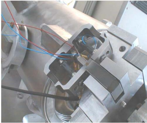
Figure 3: Close view to piezoelectric actuators in the mechanical frequency tuner.
