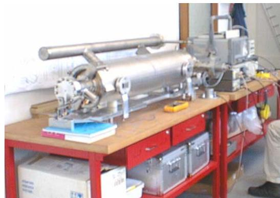
Figure 2: Experimental setup. The cavity is equipped with He tank and mechanical frequency tuner.
