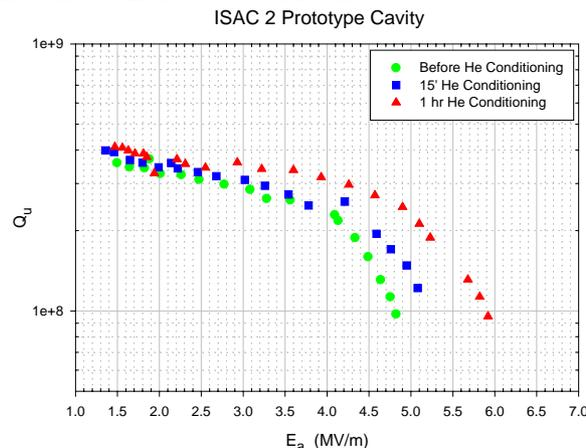
Figure 4 - Improvement in Q by Helium conditioning
