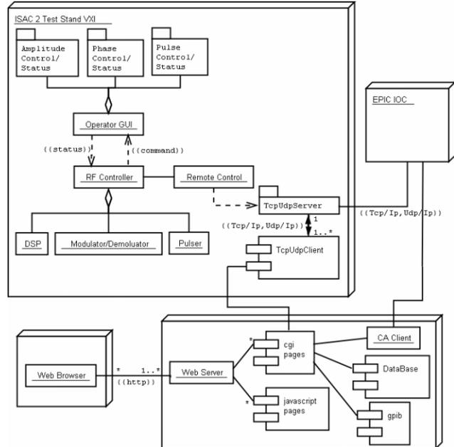
Figure 2 - Deployment Diagram of ISAC 2 Control System
