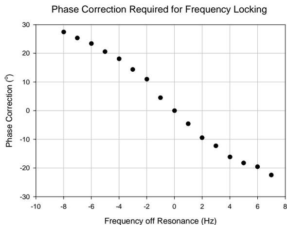
Figure 3 - Phase Correction Required for Frequency Locking
