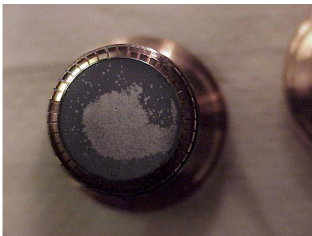
Figure 3. Copper cathode after removal from the RF gun. The cathode surface had been coated with tellurium prior to use.
