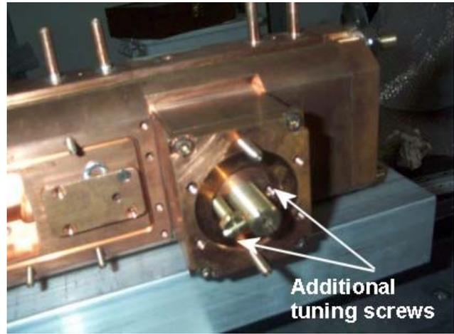
Figure 7: First SCDTL module on RF bench
