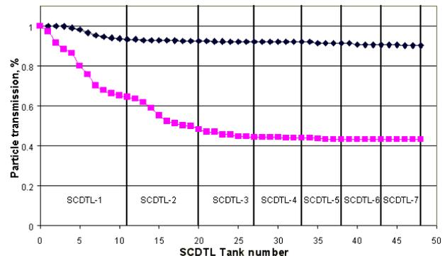
Figure 4: Beam transmission through SCDTL: Upper only transverse dynamics; lower total dynamics
