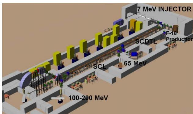
Figure 1: TOP Linac layout
