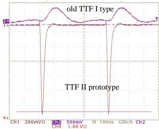
Figure 3: Signal of the prototype of the TTF II toroids together with the signal of TTF I type measured in TTF I with a bunch charge of 2.7 nC.
