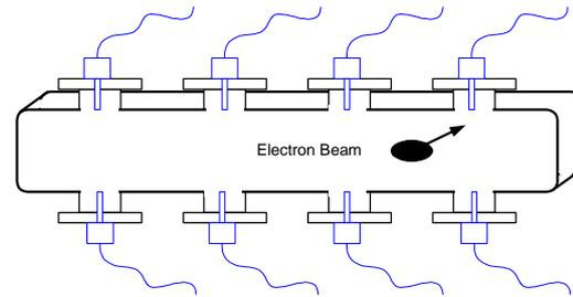
Figure 2: Schematic view of a button array for a beam pipe with high aspect ratio of the transverse dimensions typical for bunch compressors.
