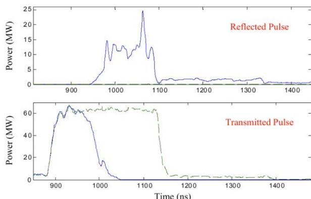
Figure 1: RF power pulse shapes during a breakdown at 11.4 GHz.
