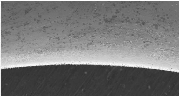
Figure 8: Direct comparison between the arc resistance of copper (upper) and tungsten (lower). The tungsten iris is shown with a higher magnification.
