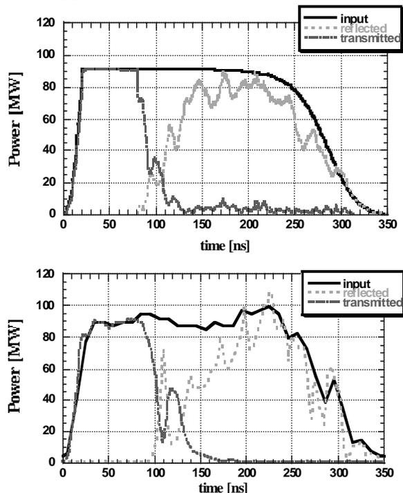
Figure 7: Measured RF signals from an 11 GHz waveguide breakdown is shown in the upper plot. Computed 11 GHz waveguide breakdown is shown in the lower plot.
