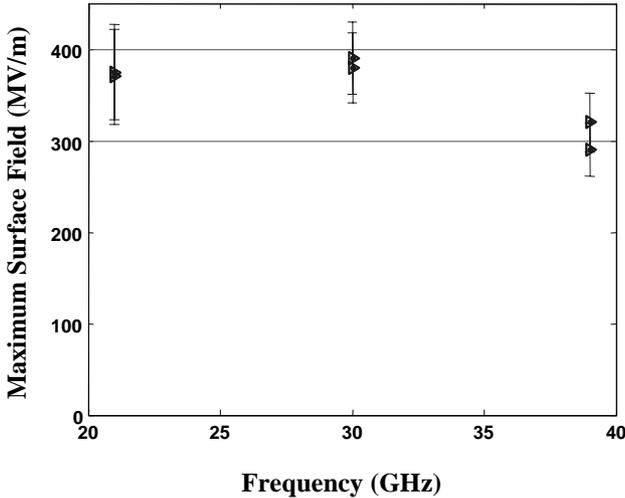
Figure 4: Final maximum surface electric field as a function of frequency achieved in six scaled single cell cavities.
