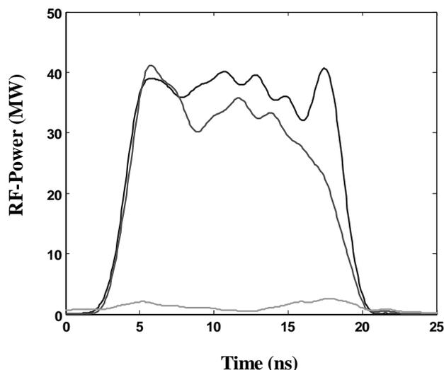
Figure 2: RF power pulse shapes during a breakdown at 30 GHz. The incident power is shown in blue (highest trace), transmitted power in red (middle trace) and reflected power in green (lowest trace).
