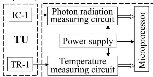
Fig. 2: Block-diagram of measuring channel
