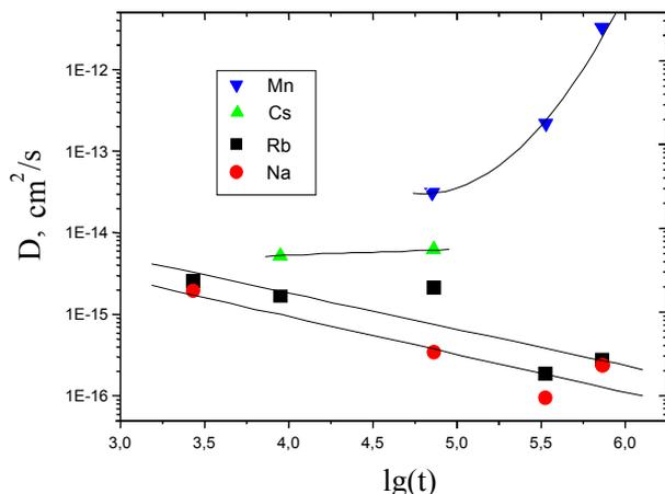
Fig. 4: Coefficients of diffusion of alkaline elements and Mn
