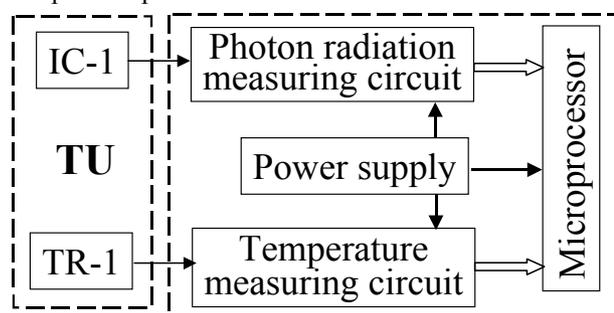
Fig. 2: Block-diagram of measuring channel
