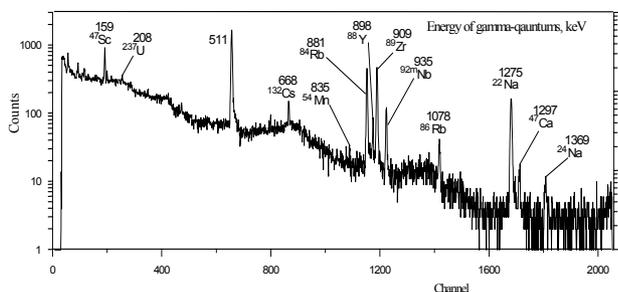
Fig. 3:  $\gamma$ -spectrum of granite sample after activation by bremsstrahlung
