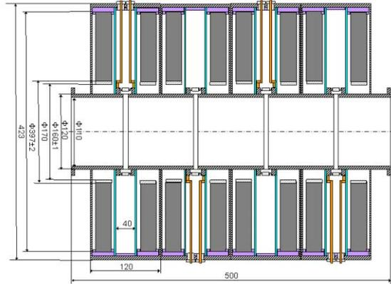
Figure 8: Multi-gap RF cavity.
