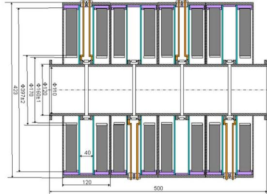
Figure 8: Multi-gap RF cavity.
