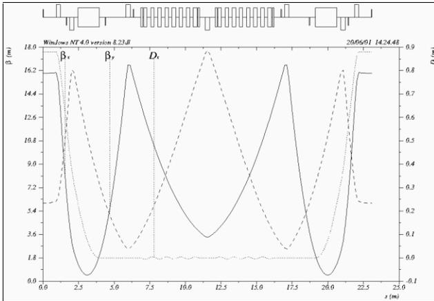
Figure 1: Lattice functions in the wiggler section.
