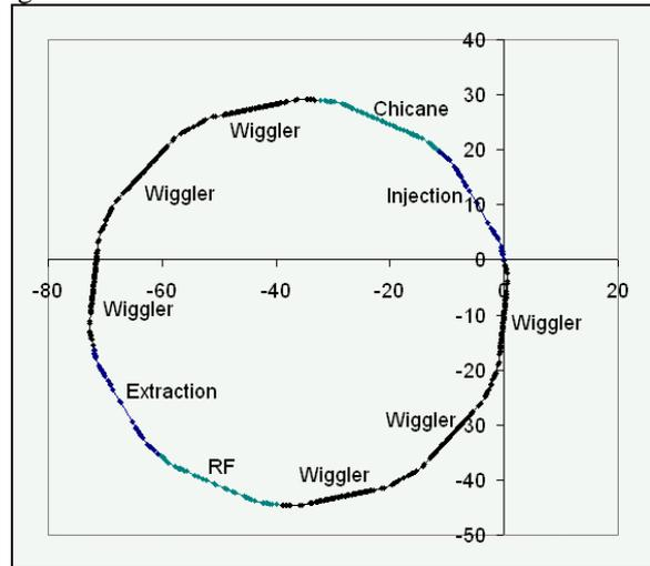
Figure 3: Pre-damping ring structure. Horizontal and vertical scales are in metres.
