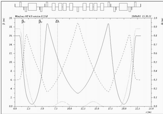
Figure 2: Lattice functions in the chicane section.
