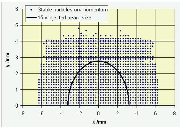
Figure 4: Dynamic aperture for on-momentum particles.
