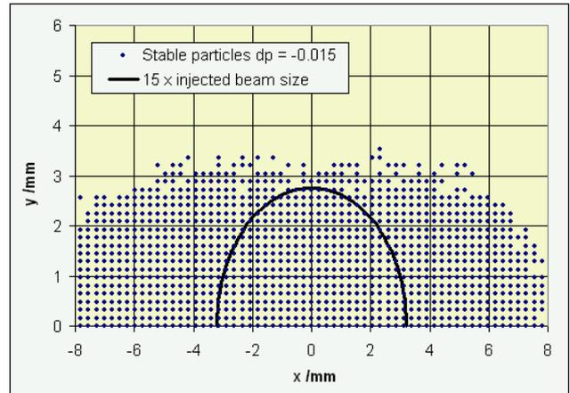
Figure 5: Dynamic aperture for particles with  $-1.5\%$  momentum deviation.
