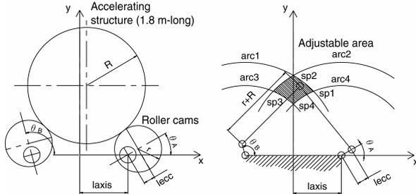
Fig 5: Conceptual roller cams mover positioning system.
