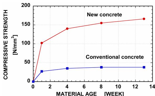
Figure 2: Comparison of the compressive strength of the new and conventional concrete as a function of material age. The new concrete provides 4.4 times higher compressive strength than conventional concrete at 13 weeks.
