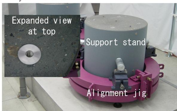
Figure 4: Full size support stand and attaching alignment jig were developed by Takenaka Co. The surface roughness and flatness are within ±10 μm.
