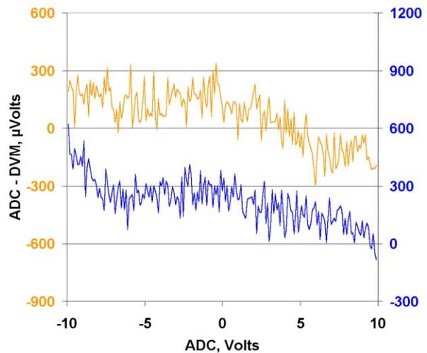
Figure 5. Linearity Results - Channels 3 and 4
