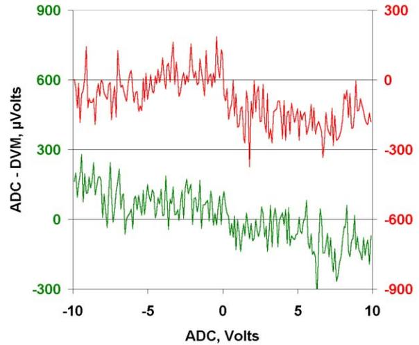
Figure 4. Linearity Results - Channels 1 and 2
