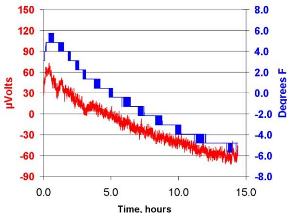
**Figure 6. DAC Temperature Stability**
