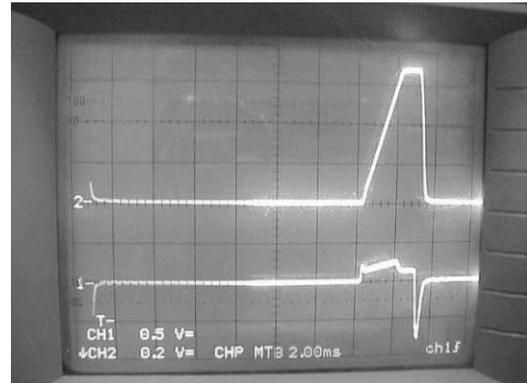
Figure 7 Experimental output voltage (375V/div) and rated output current (450A/div) with dc bias of 20A
