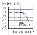
Figure 3: Nonlinearity of magnetisation curves, left: MSIB01, right: MSDC01
