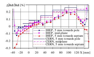
Figure 4: Transverse field homogeneity of MSIB01
