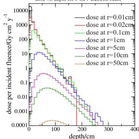
Figure 3: Annual dose rate induced by 3 GeV electron beam in ordinary concrete (CCT).
