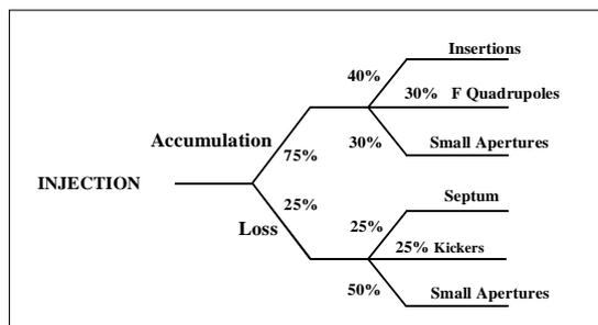
Figure 2: Diagram of the expected electron beam losses in CANDLE (“top-up” mode).
