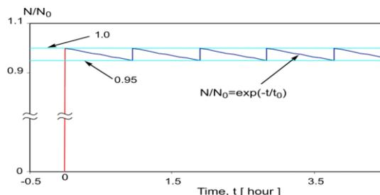
Figure 1: The stored beam time structure in “top-up” injection mode.
