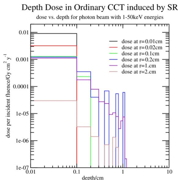
Figure 4: Downstream dose distribution for CANDLE shielding (ordinary concrete).
