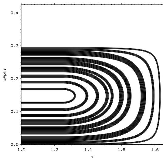
Fig. 4. End-turn layout on the developed winding cylinder with the shape function of Fig. 1, the 2-D design of Table I, and the block group definition of Table II, showing individual turns.
