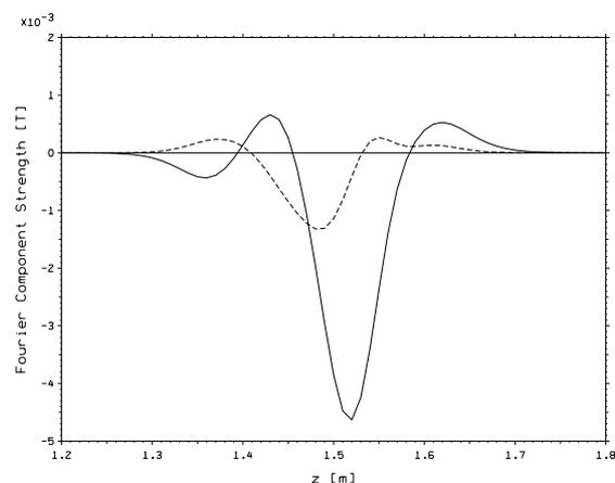
Fig. 5. Plot of the  $m=6$  (solid curve) and  $m=10$  (dashed curve) Fourier components of  $B_r$  in the end region of magnet. The straight part of the windings ends at  $z = 1.325$  and the end of the windings is at  $z = 1.625$ .
