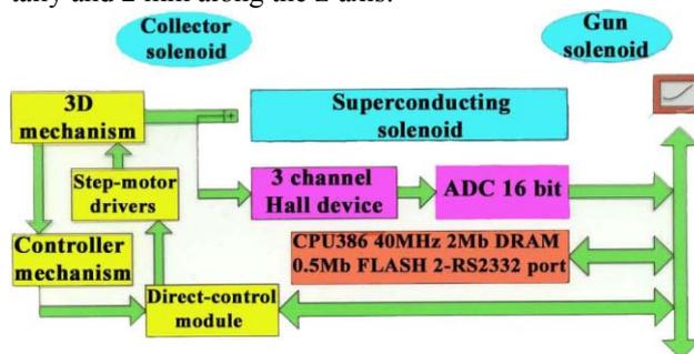
Fig. 2. Block diagram of the 3D Hall measurement system.
