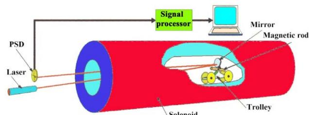
Fig. 3. Schematic drawing of the process to trace the magnetic field lines in the main solenoid. The actual trolley supports a small rod-mirror assembly in a compound gimbal.
