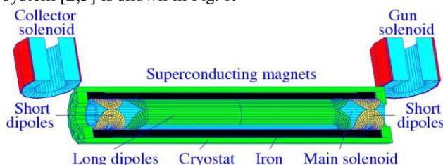
Fig. 1. Longitudinal cross-section of the magnetic system.
