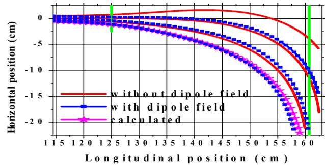
Fig. 5. Magnetic lines from the SC solenoid to the collector one.
