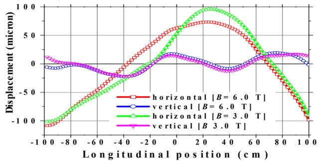
Fig. 6. Transverse displacement of various field lines along the length of the main solenoid at different field strengths.
