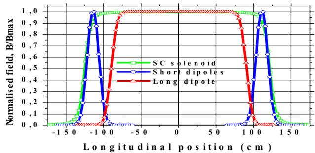
Fig. 4. Longitudinal distribution of the normalized fields of the SC magnets.
