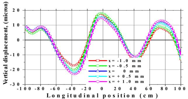
Fig. 7. Transverse displacement of various field lines along the length of the main solenoid at different horizontal positions.
