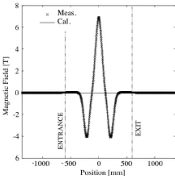
Fig. 4 Magnetic field distribution of the prototype wiggler.
