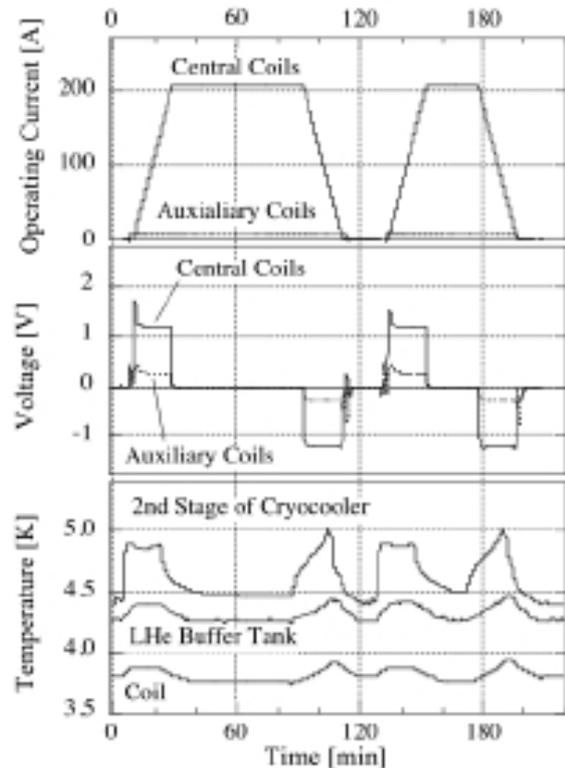
Fig. 3 Coil voltages and temperatures at some points for Current operation.
