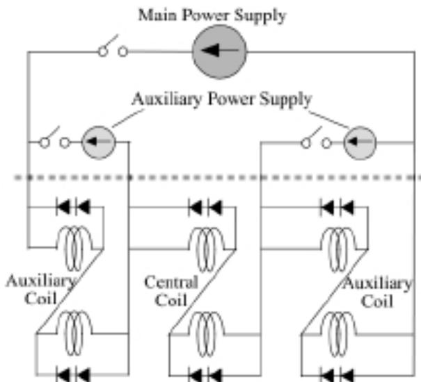
Fig. 2 Circuits of the prototype wiggler.
