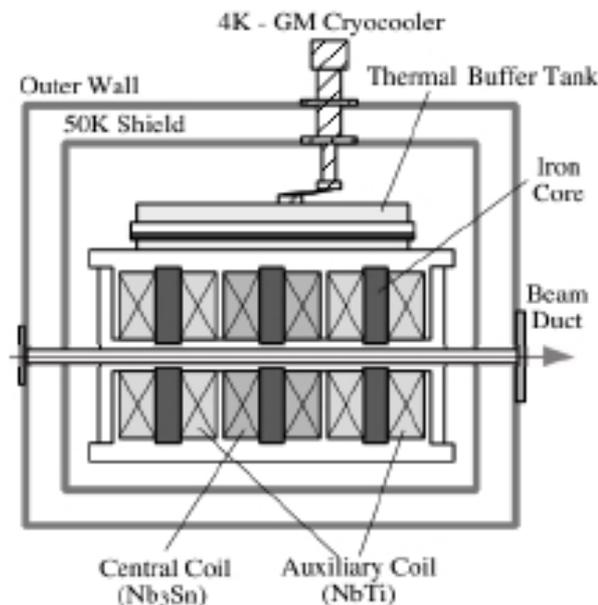
Fig. 1 Schematic view of the prototype wiggler.
