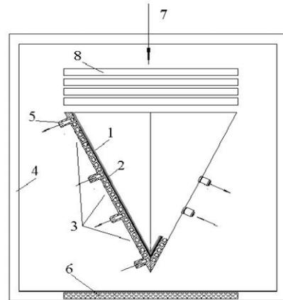
**Figure 2:** Layout of conical target with liquid agent cooling. 1 – operation layer, 2 – liquid metal layer, 3 – blanket with cooling channels, 4 – vacuum chamber, 5 – inlets and outlets of cooling channels, 6 – neutron beam output window, 7 – primary beam, 8 - collimator.
