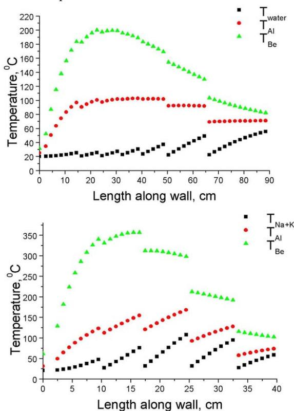
**Figure 3:** Operation layer, cooling channel wall and coolant temperature along cone wall. Above - water cooling, below - Na+K cooling.
