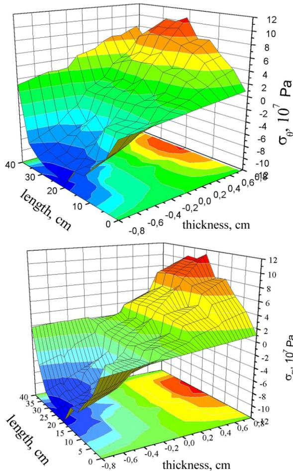
**Figure 4:** Azimuth (above) and meridian (below) thermo-mechanical stress distribution ( $10^7$  Pa) over the cone length and thickness. Operation layer - Be, blanket - Al, coolant - Na+K
