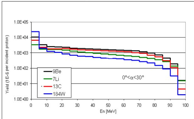
**Figure 1:** Comparison of neutron production yield in different converters, in the forward direction
