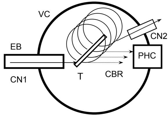
Figure 1. The scheme of experimental setup. VC is a vacuum chamber, T is a crystalline target immersed in a magnetic field, EB is an electron beam, PHC is photon channel for CBR, CH1 and CH2 are channels for injection and removal of electrons.
