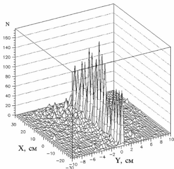
Figure 2. Spatial distribution of intersection points of circling electron trajectories with a target plane (demonstration test with the increased step of cross drift of 5 – MeV electrons in 30 mkm silicon target; ). X-axis is vertically directed; Y-axis is stretched along a target.
