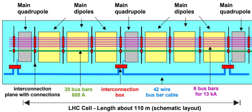
Figure 3: Layout of a LHC Cell including bus bars
