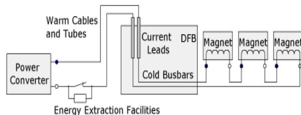
Figure 2: Typical electrical circuit in the LHC
