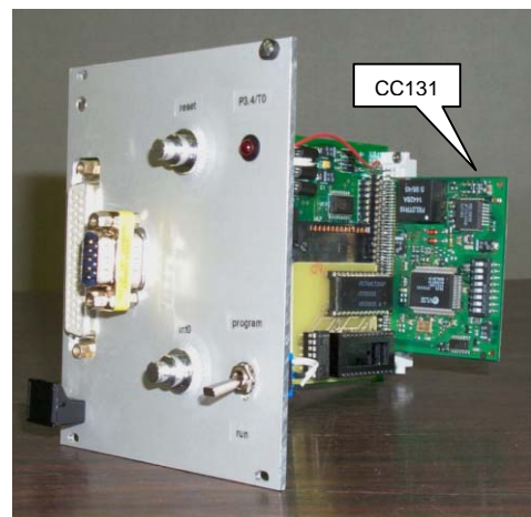
Figure 2 : Physical view of the WorldFIP node showing the ALSTOM's CC131 module.
