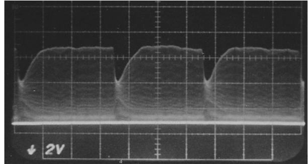
Figure 1: Vertical beam size versus time showing emittance blowup caused by ion trapping in the KEK photon factory (courtesy S. Sakanaka).
