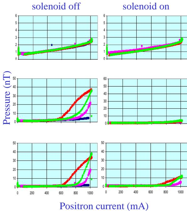
Figure 10: Pressure versus total positron current at PEP-II in the arcs (top), the start of a straight section (middle), and in the middle of the straight (bottom) with and without a solenoidal confinement field. The different curves correspond to bunch spacings of  $\tau_d$  (black star),  $2\tau_d$  (pink square),  $3\tau_d$  (red triangle), and  $4\tau_d$  (green diamond), where  $\tau_d$  is the design bunch spacing.
