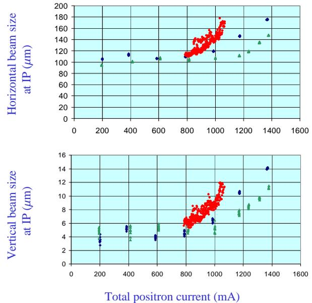
Figure 11: Beam size at the PEP-II interaction point measured with a single beam without solenoids (blue diamonds), with a single solenoid (green triangles), and with beams in collision (red circles).
