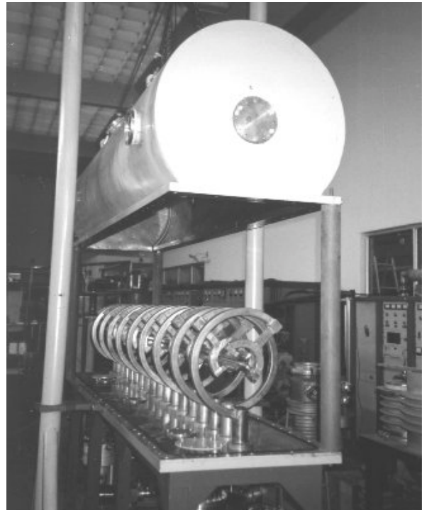
Figure 6: The ISR RFQ-1000 resonator
