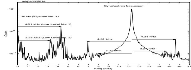
Figure 5: Beam signal spectrum at 236.6 mA, 2.04 GeV when two kind noises are generated simultaneously.
