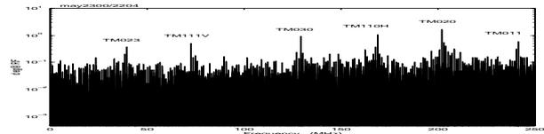
Figure 3: Pseudo-spectrum when LFS is turned off at 203.0 mA, 2.04 GeV. Four cavity temperatures are 40.8°C, 46.8°C, 45.6°C, and 36.9°C, respectively.
