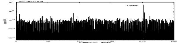
Figure 2: Pseudo-spectrum of 468 bunches (b) when the LFS is turned off at 161.9 mA, 2.5 GeV. Four cavity temperatures are 37.8°C, 47.2°C, 45.7°C, and 38.1°C, respectively.
