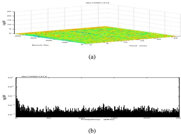
Figure 1: Time domain 400-bunch oscillations (a) and their pseudo-spectrum (b) when the LFS is turned on at 165.3 mA, 2.04 GeV. Four cavity temperatures are 37.8°C, 47.3°C, 45.7°C, and 37.8°C, respectively.
