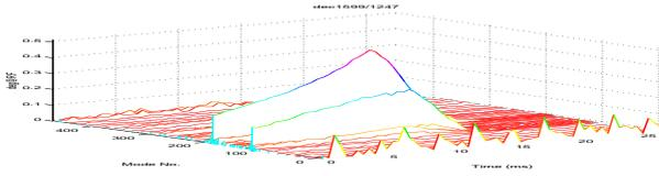
Figure 4: Evolution of two modal strengths in the frequency domain when the grow/damp process for 400 bunches is performed by the LFS at the beam current of 153.1 mA, 2.04 GeV. Temperature status is the same as that of Fig. 1.
