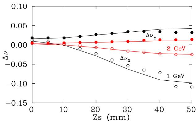
Figure 2: Horizontal and vertical tune shifts induced by EU10.0 at 2.0 and 1.0 GeV
