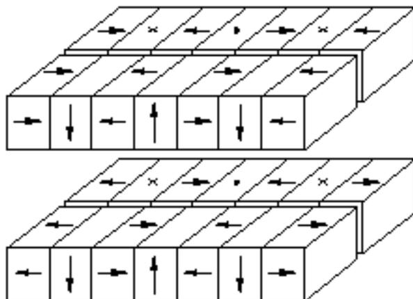
Figure 1: Schematic layout of an APPLE-2 undulator
