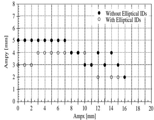
Figure 3: Comparison of dynamic aperture simulations at 2.0 GeV with and without the elliptical undulators in circularly polarized mode.
