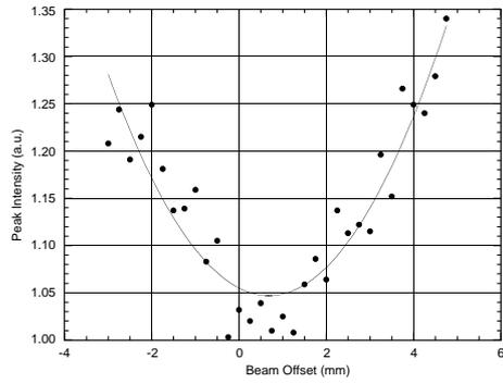
Figure 5: Radiation intensity versus the beam position.
