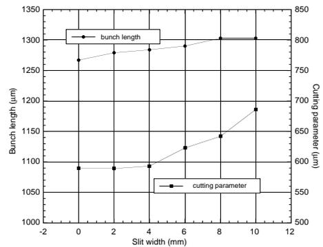
Figure 7: The bunch length and the cutting parameter versus the slit width.
