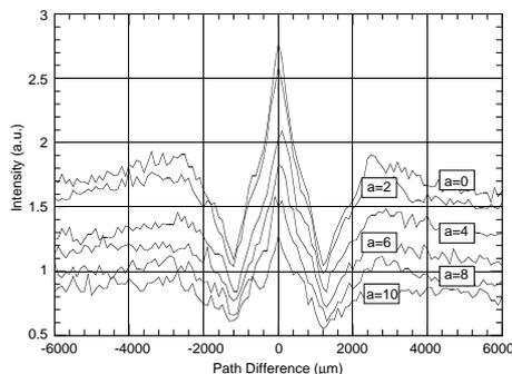
Figure 2: The detector signal as a function of the optical path difference for different slit widths.
