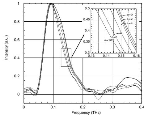
Figure 3: Normalized coherent radiation spectra for different slit widths.
