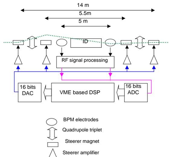
Figure 3: The local feedback principle
