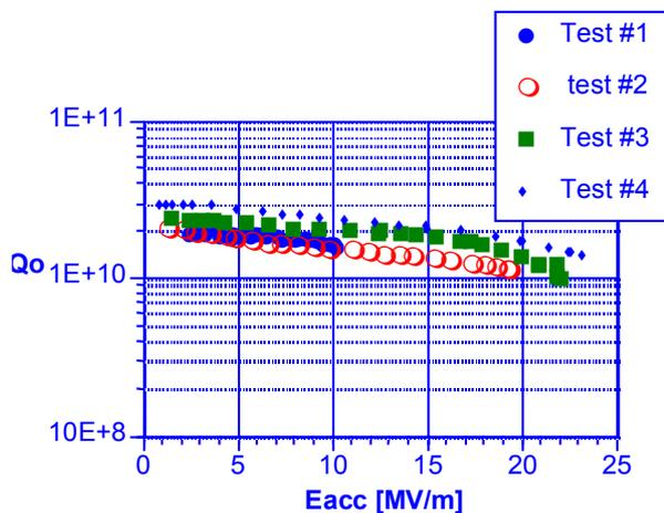
Figure 2: Results for cavity 1BT1; test #1: 40  $\mu$ m bcp, test #2:  $\approx 80$   $\mu$ m bcp, test #3 :  $\approx 105$   $\mu$ m bcp, test #4:  $\approx 135$   $\mu$ m bcp.
