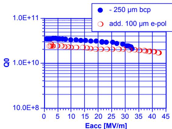
Figure 3: Q vs Eacc for cavity 1K2 after bcp and ep surface treatment.
