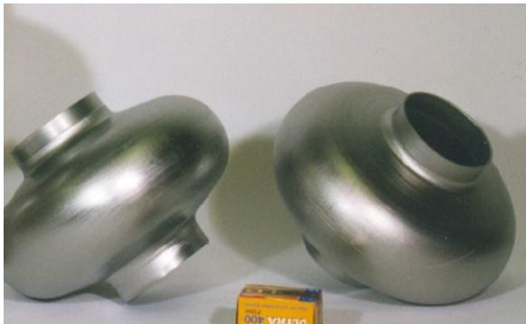
Figure 1: Mono cell cavities fabricated at DESY.
