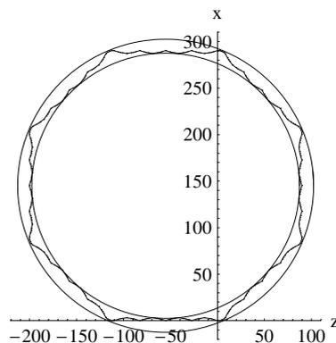
Figure 3: Geometry of the isochronous, thin lens, FODO lattice with wigglers. The inner and outer circles represent the walls of the existing ISR tunnel
