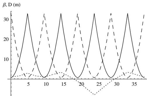
Figure 2: Optical functions for the isochronous, thin lens, lattice with wigglers ( $\beta_h$  solid,  $\beta_v$  dashed,  $D_h$  dotted line). A single FODO cell with half wiggler cell is shown.
