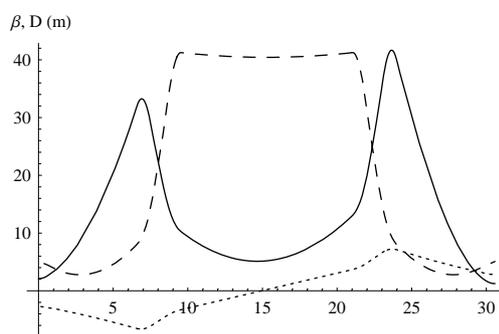
Figure 4: Optical functions for half a super-period of the isochronous, thick lens, lattice with negative curvature dipoles ( $\beta_h$  solid,  $\beta_v$  dashed,  $D_h$  dotted line).
