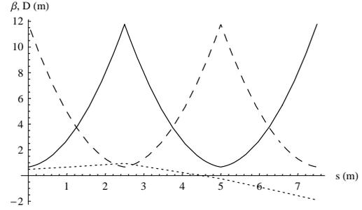
Figure 1: Optical functions for half a wiggler module with two parameters ( $\beta_h$  solid,  $\beta_v$  dashed,  $D_h$  dotted line). In this case  $\psi = 0.03$  rad,  $f = 1.4$ ,  $L = 5$  m.
