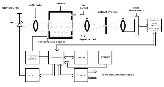
Fig.2. Liquid level optoelectronic sensor lay-out.
