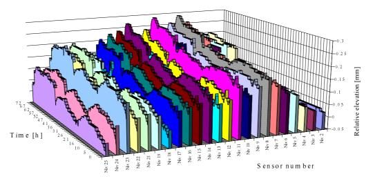
Fig.4. The relative elevation of measured Nuclotron magnets
