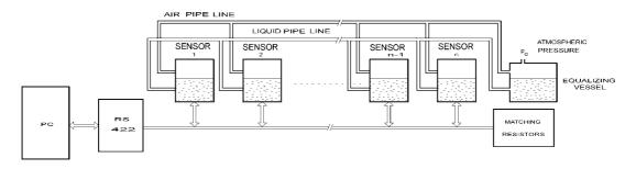
Fig.1. A block-diagram of hydrolevelling system.
